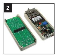
The separated halves appear as above. The PCB of interest is the auxiliary PCB, shown on the right half, adjacent to the battery. Remove the battery before beginning work on the modifications.
