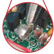
Using a pair of wire cutters, cut the connection between the components.
