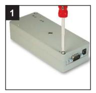
Separate the two halves of the gauge housing by loosening the captive screws. Then pull the two halves apart.
